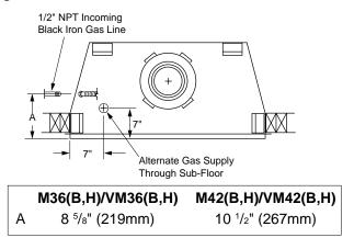
Figure 19 - Routing Incoming Gas Line
